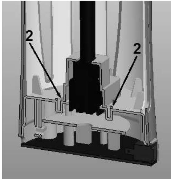
The light socket is under the covering cap (1). This cap is fastened to the base with 2 screws (2). To replace the light hold the lid of the Glue trap, use a screwdriver to unscrew both plugs and remove the cap. You can now easily pull the light out of the socket in order to replace it. Finally, refit the cap and fasten it with the screws. Only use the same type of light!
